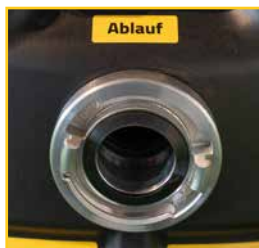
C-coupling suitable for fire hoses
